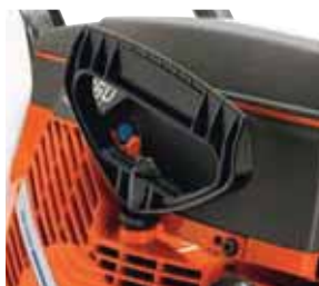
Specially designed starter handle.
